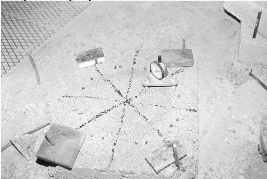
Figure 3. Gauge depth measurement in abrasion resistance test
