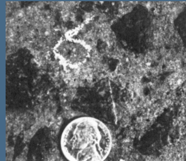
Polish coarse aggregates contributes to low skid resistance
