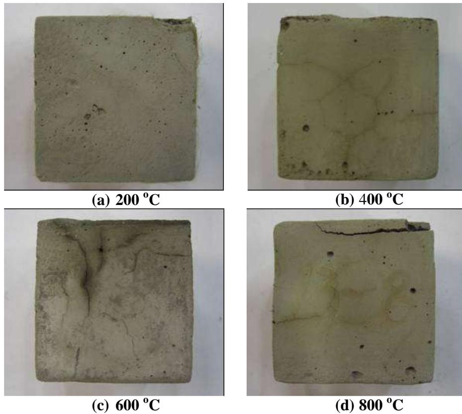
**Figure 3. Typical crack patterns on the surface of ECC cubic specimens after exposure to high temperatures**
