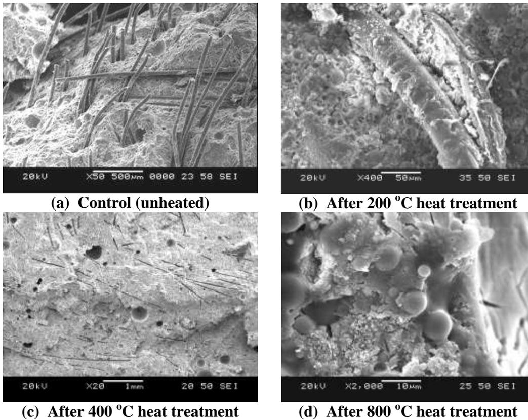
**Figure 2. SEM micrograph before and after thermal treatment**
