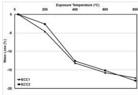
**Figure 4. Change in mass loss of ECC mixtures with temperature**
