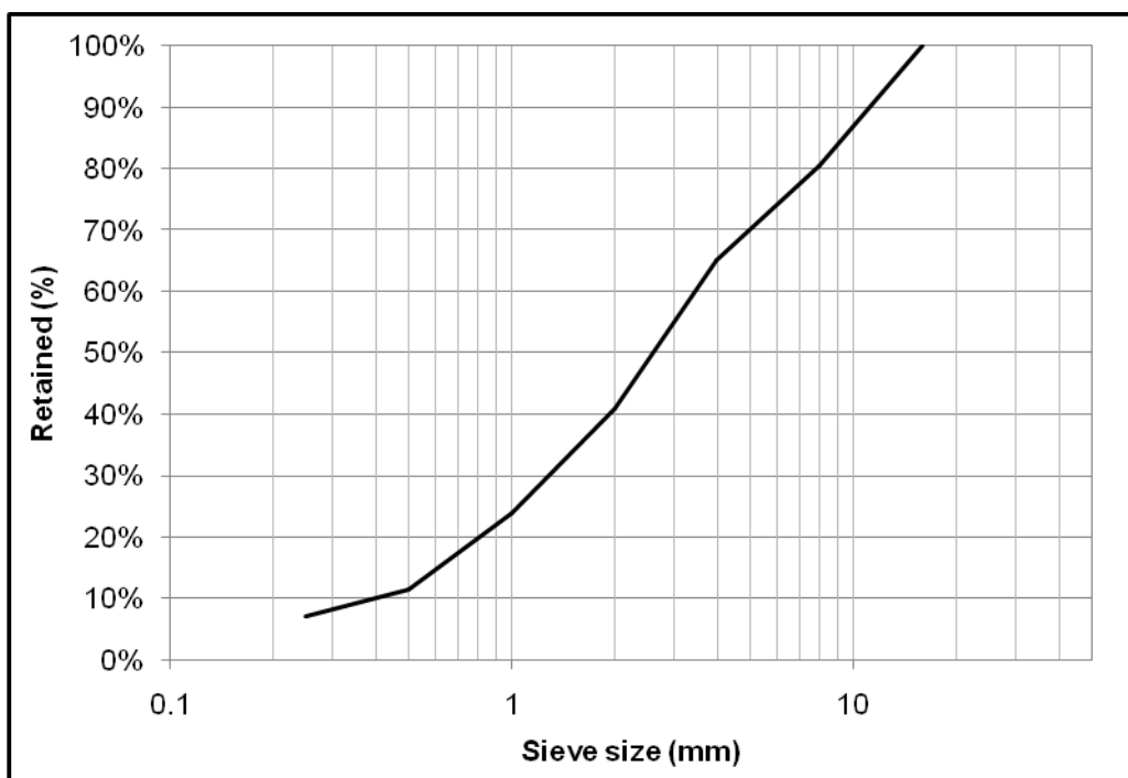
Fig. 1. Granulometry of aggregate mix used in all SCC mixtures
