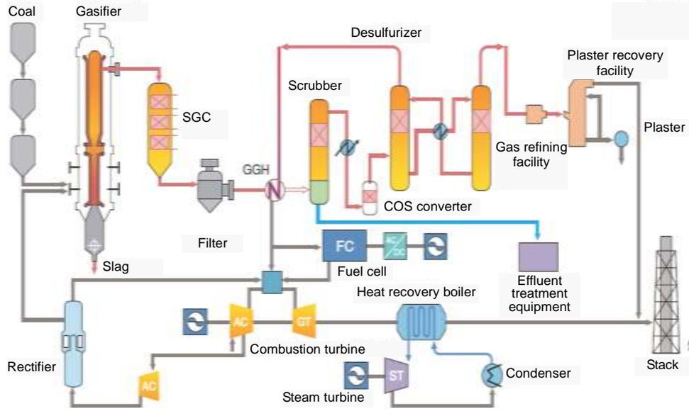
Figure 2: Structure of coal gasification unit
