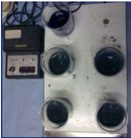
Fig. 5 (a) exposing fly ash to AB80 solution and (b) concentration determination with colorimeter
